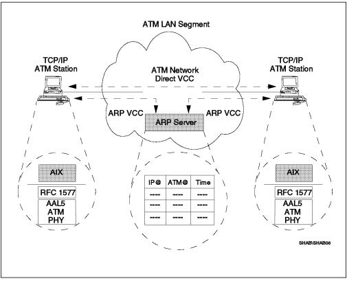
Figure 4. ATM Classical IP using ARP Server
